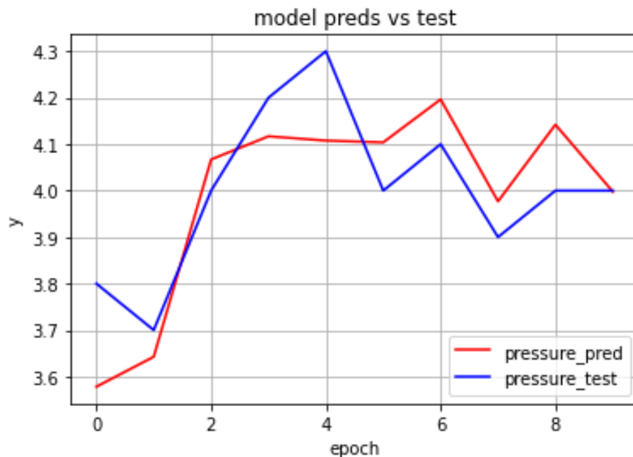
Figure 20. Pressure prediction results of the NN model compared to the actual test value.
